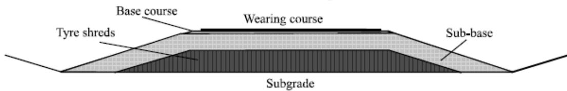
Figure 2 Embankment with tyre shreds
