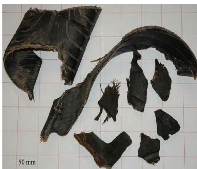
Figure 3 Fragmentation of tyre shreds
